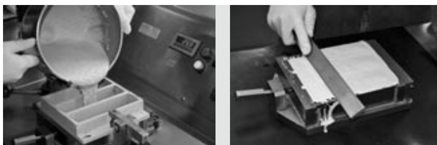
Fig. IV-7: Testing super-sulfated cement according to prEN 15743 – filling the mortar mould (left) and wiping off the matrix (right)
