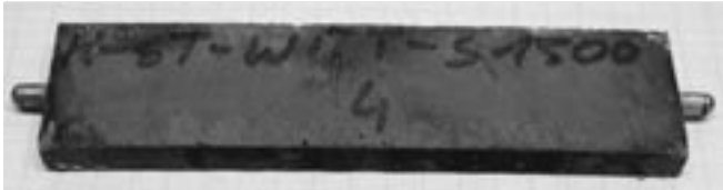
Fig. III-27: Flat mortar prism made from highly sulphate resisting Portland cement (CEM I 32.5 R - HS) after 24-month storage in sodium sulphate solution (1500 mg SO 4 /l) at 8 °C
