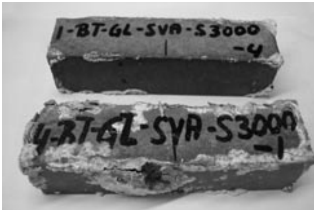
Fig. V-37: Concrete specimens (w/c = 0.60) based on Portland cement (CEM I 32.5 R) and quartz gravel (upper part of the figure) or limestone chippings (lower part of the figure) as aggregate after 40-month storage in 0.44% sodium sulphate solution at 8 °C
