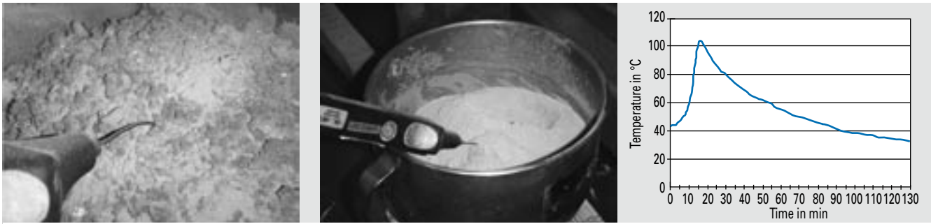
Fig. IV-9: Trials on the pre-slaking of a road binder containing quick lime: appearance of the road binder immediately after mixing (left) and after the slaking process was completed (middle) as well as temperature development during the slaking process (right)
