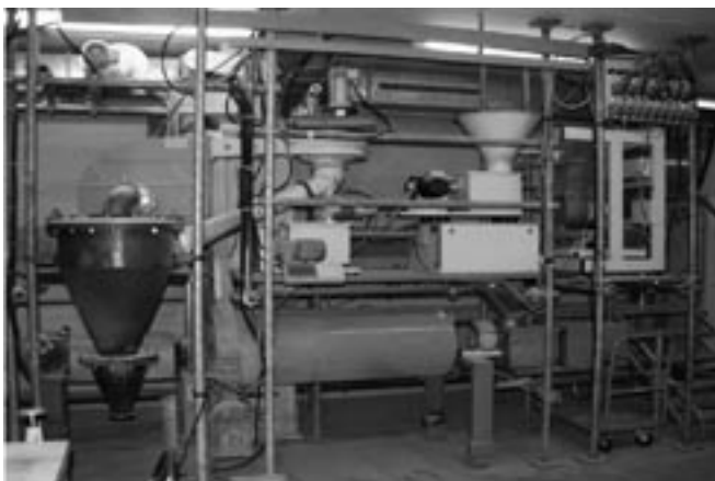
Fig. I-27: Semi-industrial ball mill of the Research Institute
