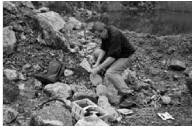
Fig. V-38: Concrete cubes wrapped in wide-meshed plastic gauze prior to storage in the lake saturated with gypsum water that can be seen in the background
