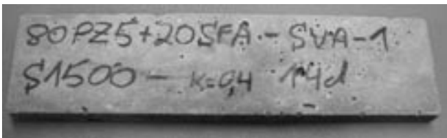
Fig. III-31: Flat mortar prism made from a mix consisting of 80 mass % CEM II/A-LL 32.5 R and 20 mass % CFA (k = 0.4) after 24-month storage in sodium sulphate solution (1500 mg SO 4 /l) at 8 °C
