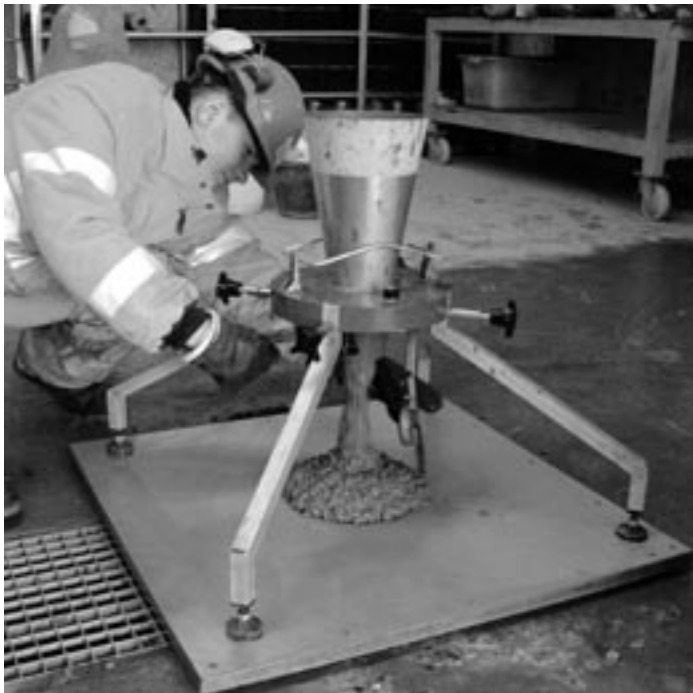
Fig. V-44: On-site use of the VDZ flow cone for determining the fresh concrete properties of SCC
