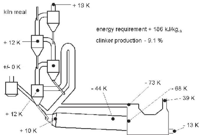
Figure 2: Effect of low dust collection efficiencies in the preheater
