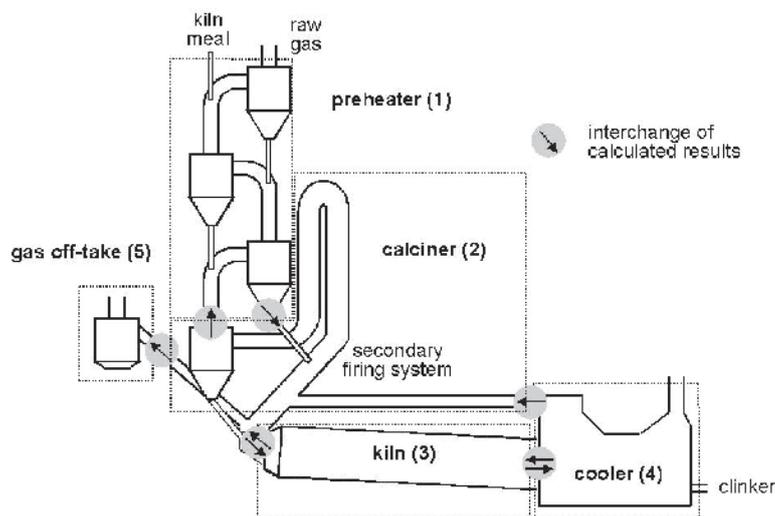
Figure 1: Balance areas and calculation sequence for the plant sections
