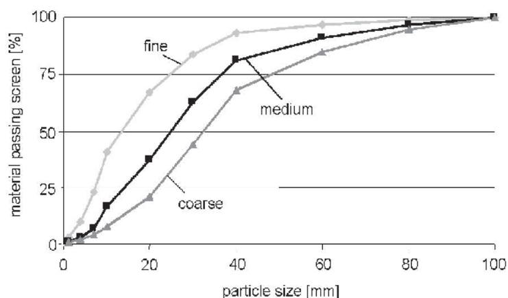
Figure 3: Particle size distribution of the clinker
