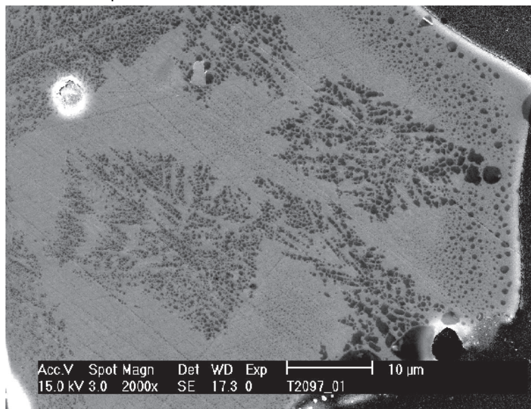
Figure 8: The picture using secondary electrons reveals the surface structure clearly. In the crystalline edge zones, an increased porosity becomes discernible.
