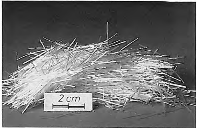
Bild 12 Fasern aus E-Glas (Bor-Silicat-Glas)
