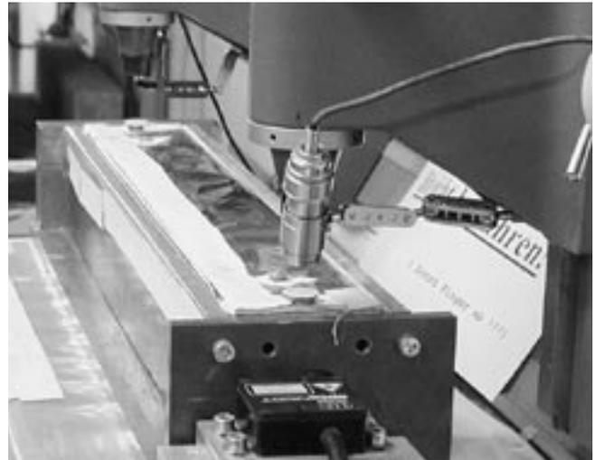
extensometer, using test marks made 400 mm apart on the surface of the test piece. After 105 days the test piece was removed from the special steel foil and stored at 20 °C and 65 % r.h., and the shrinkage measurements were continued.
